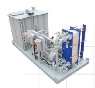
In normal drilling operations excess heat is produced by the braking system used at the drawworks, winches and mooring systems. The Brakes can absorb thermal loads generated by applying torque; this thermal load must be dissipated by using Cobra's custom designed "Brake Cooling System". These systems are engineered to provide proper cooling dissipation and can be configured to meet any footprint requirement.
