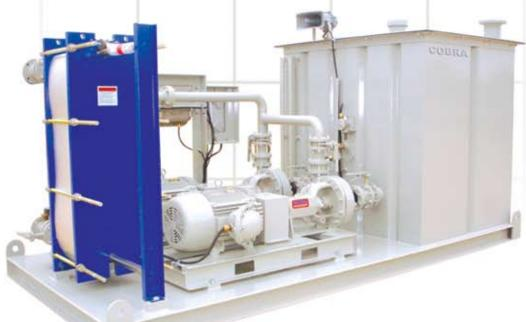
Cobra manufactures a range of custom break water cooling systems to suit individual customer requirements.
